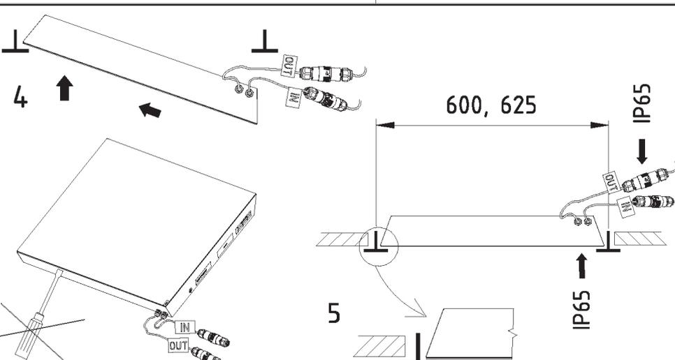
4. Mount the luminaire to the ceiling using the provided screws.
