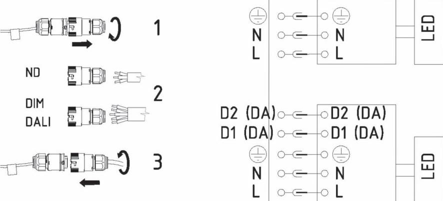
1. Connect the main power cable (OUT/IN) to the LED module terminals (N, L).
